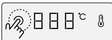
To check the current temperature of the food, press the touch area on the digital panel.
